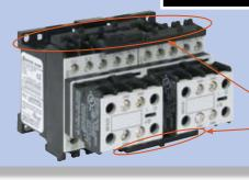
The Printed Circuit Board Link Module installs directly on the terminals of standard mini contactors and control relays enabling them to be directly mounted on an electronic printed circuit board. The module is rated 16A AC-3 and 22A AC-1 to take full advantage of the maximum switching capability of the mini contactor and control relay.
