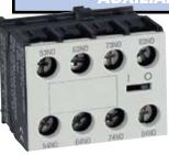
Our front mounted auxiliary contact modules feature IP20 guarded terminals to protect against accidental contact with live parts. The modules are available in 2 and 4 circuit configurations. The device identification marker simplifies trouble shooting in panels with many devices. These modules snap-on and install without the use of tools. NOTE: See chart below for maximum number of front mounted auxiliary contacts.
